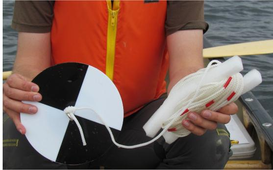
**Figure 10.** Disque de Secchi (photo Michel Grégoire, 2014)
